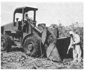
PLUTONIUM in the top soil is scraped up by bulldozers, mixed with concrete and dumped into a restricted are. Few areas remain where anti-C suits are needed.
